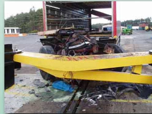
The Terra Road Closer being successfully crash tested, stopping a 7500kg lorry travelling at 80kph
