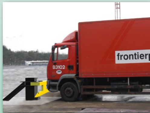
The Terra Road Closer being successfully crash tested, stopping a 7500kg lorry travelling at 80kph
